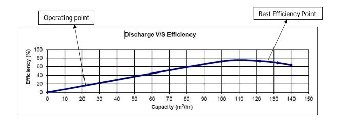
From the characteristic curve shown, it can be seen that the best efficiency point of the pump is between 122 to  $132 \, \text{m}^3/\text{hr}$  flow. The observed flow is  $21.25 \, \text{m}^3/\text{hr}$  which indicates the operating point is far away from the best efficiency point.
